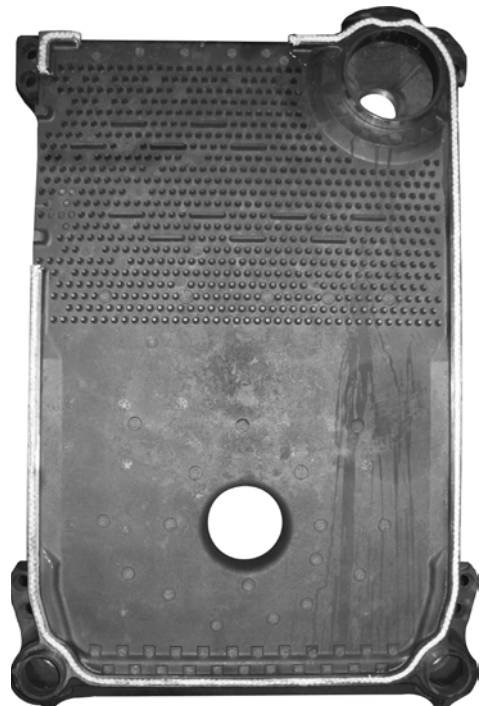
Figure 7: Affixing the Fiberglass Rope
