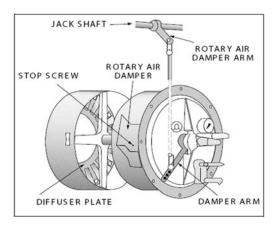
monthly. If necessary, tighten the setscrews and the connections at the uniballs. Check the uniballs for wear and replace if necessary. The linkage assembly should be tight but should not bind. If the
