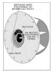
There are relatively few adjustments that can be made to the burner, however, a check should be made to assure that all components are properly located, and that all holding screws are properly tightened.
