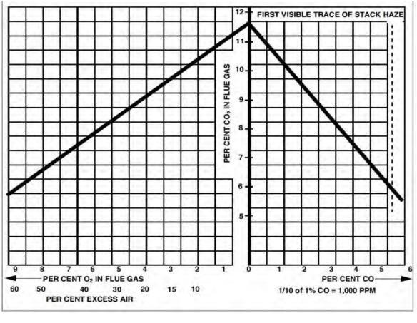
FIGURE 6-14. Flue Gas Analysis Chart for Natural Gas
