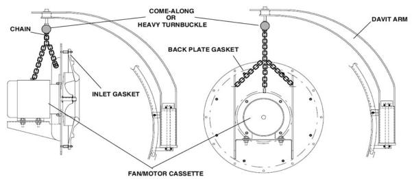
NOTE: 400-800 HP RECOMMEND USING A 3-POINT DAVIT ATTACHMENT FROM THE DAVIT ARM TO THE FAN / MOTOR CASSETTE
