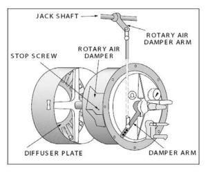
FIGURE 6-2. Rotary Air Damper
