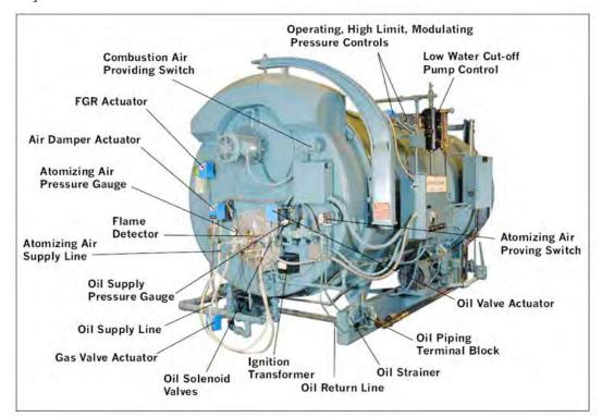
FIGURE 2-4. Steam Boiler Components and Controls
