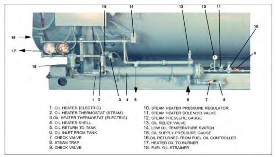
FIGURE 2-11. Oil Heating Assembly (Steam)
