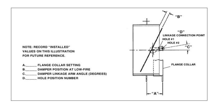
FIGURE 5-15. Flange Collar and Damper Settings (Top View)
