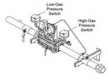
FIGURE 6-16. Gas Train Pressure Switches
