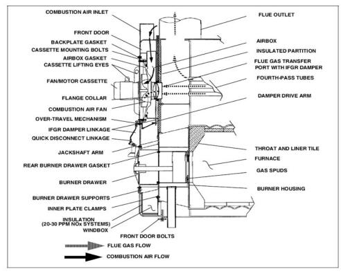
FIGURE 1-11. Cross Section of Front Head
