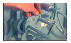
FIGURE 5-5. Oil Gun Locked in Firing Position
