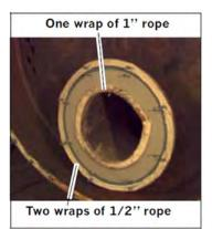
Swing the door to the closed position and run all retaining bolts in until snug. Tighten the bolts uniformly, starting at the top center and alternating between the top and bottom bolts until both are tight. Do not over-tighten. Tighten alternate bolts until all are secure and the door is gas tight.
