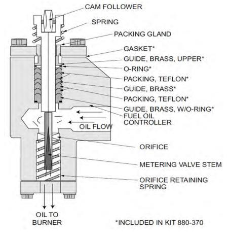
FIGURE 8-27. Fuel Stem Packing, Cross-Section
