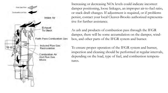
FIGURE 8-22. Induced Flue Gas Recirculation (IFGR) Air Flow
