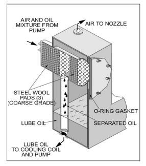
Air pressure from the pump also forces sufficient oil from the tank to the pump bearings to lubricate them and also to provide a seal and lubrication for the pump vanes. As a result, the air delivered to the tank contains some lube oil; however, most of it is recovered through baffles and filters in the tank before the air passes to the burner.
