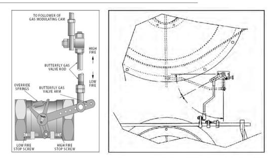
FIGURE 1-12. Over-Travel Mechanism and Fuel Changeover Linkage
