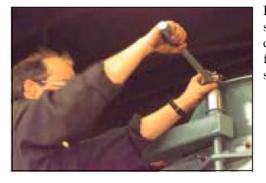
Before opening the doors, tighten the nut on the davit arm to create slight tension. This will minimize sagging and facilitate opening of the door. After opening either door, check the gaskets and seating surfaces. Replace the door gaskets if they are hard or brittle. Clean the sealing surfaces of the door and tube sheet.
