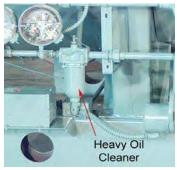
Keep the cartridge of the oil strainer clear by regularly giving the exterior handle one complete turn in either direction. Do this often until experience indicates cleaning frequency necessary to maintain optimum conditions of flow. If the handle turns hard, rotate the handle back and forth until it can be turned through a complete revolution. Do not force it with a wrench or other tool.
