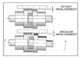
Alignment of the pump and motor through the flexible coupling is extremely important for trouble free operation. Check the coupling alignment semi-annually and replace the coupling insert as required. Keep the coupling guard in place.
