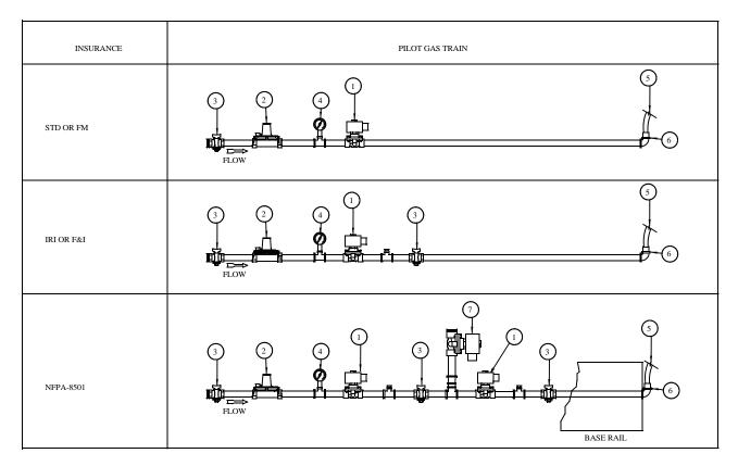
RELIEF VALVE REQUIRED ON CSD-1 WHEN SUPPLY PRESSURE IS GREATER THAN 5 PSI.
