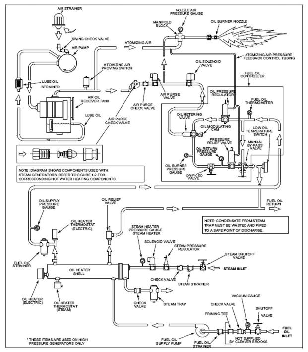
FIGURE 2-17. Diagram for No. 6 Heavy Oil Flow (Steam-Electric Heater)
