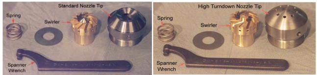
FIGURE 8-14. Standard and High Turndown Burner Nozzle Components
