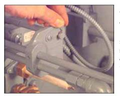
FIGURE 5-11. Oil Gun in the Lock-Out Position
