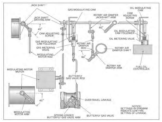
FIGURE 6-1. Complete Linkage Assembly: Combination Gas and Oil
