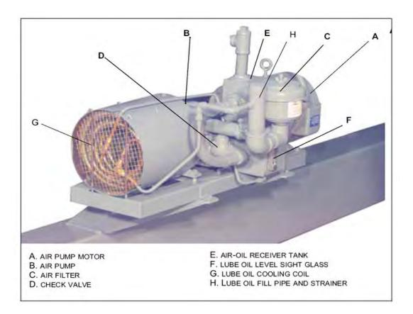
FIGURE 2-10. Air Pump (Primary Air)
