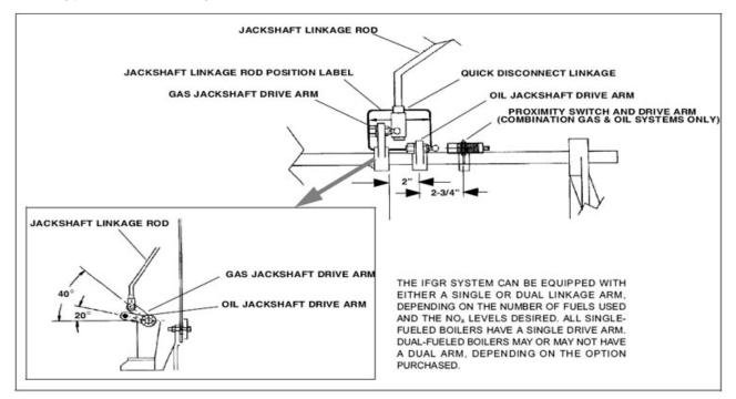
FIGURE 5-13. Jackshaft Linkage Settings
