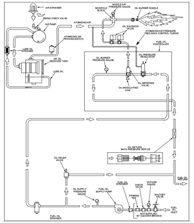
FIGURE 2-16. Diagram for Light Oil Flow
