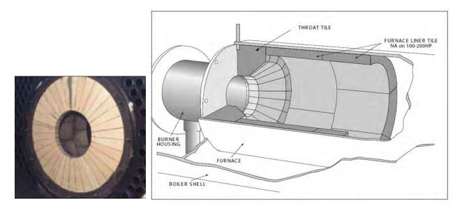
FIGURE 8-32. Throat Tile and Furnace Liner
