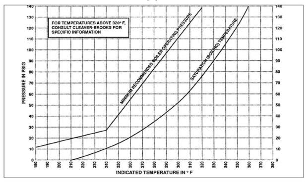
FIGURE 3-3. Internal Boiler Pressure
