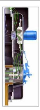
The low emission option for the CBEX Elite line of Firetube Boilers reduces Nitrogen Oxide (NOx) emissions, a major contributor to ozone pollution (smog). Carbon Monoxide (CO) emissions also tend to be lower as increased turbulence caused by the addition of the flue gases into the combustion air stream results in improved combustion.
