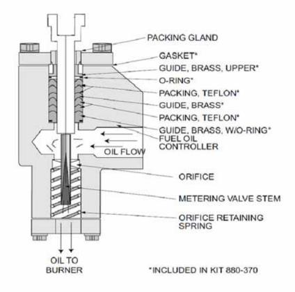
FIGURE 8-15. Fuel Stem Packing, Cross-Section
