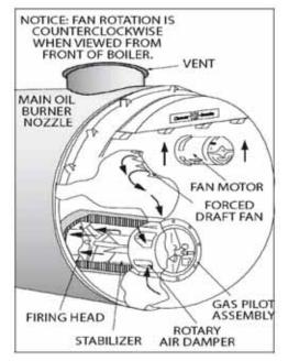
FIGURE 2-5. Secondary Air Flow Diagram
