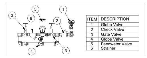
FIGURE 3-4. Feed piping, typical
