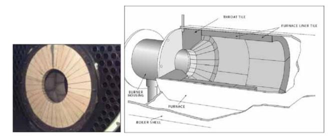
FIGURE 8-19. Throat Tile and Furnace Liner
