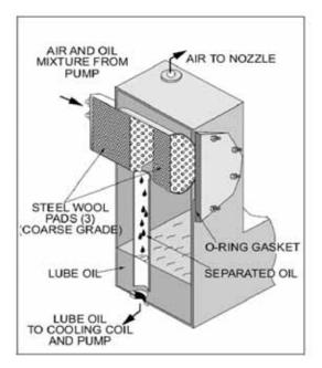
Air pressure from the pump also forces sufficient oil from the tank to the pump bearings to lubricate them and also to provide a seal and lubrication for the pump vanes. As a result, the air delivered to the tank contains some lube oil; however, most of it is recovered through baffles and filters in the tank before the air passes to the burner.
