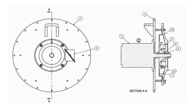
**NOTE:** Impeller size is based on boiler hp, ppm emission level, boiler operating pressure and altitude. To ensure proper application sizing, contact Cleaver-Brooks Aftermarket.
