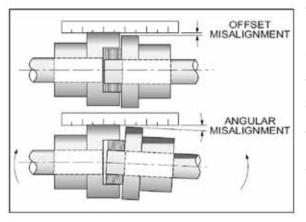
FIGURE 8-18. Flexible Coupling Alignment
