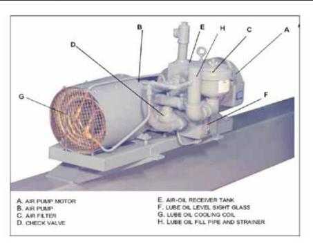
FIGURE 2-4. Air Pump (Primary Air)
