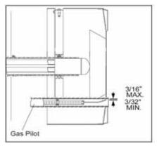
FIGURE 6-8. Gas Pilot Electrode
