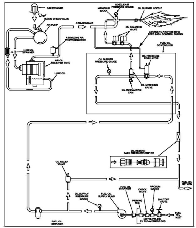
FIGURE 2-7. Diagram for Light Oil Flow
