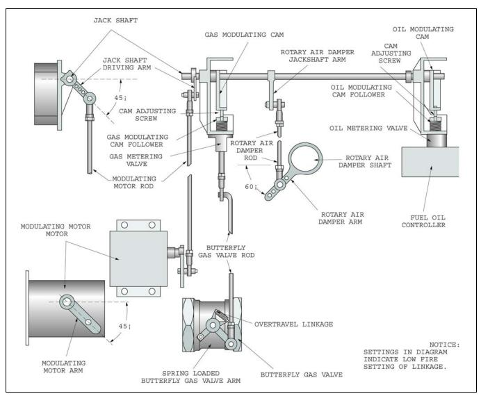
Figure 6-1 Complete Linkage Assembly - Combination Gas and Oil
