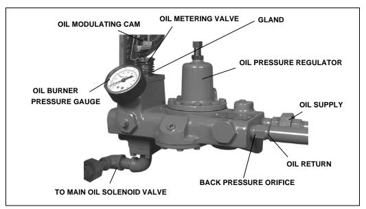
Figure 2-11 Oil Control Valve Assembly - Light Oil
