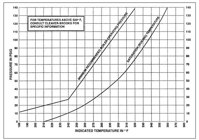
Figure 3-1 Internal Boiler Pressure
