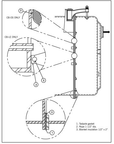
Figure 8-3 Rear door seal
