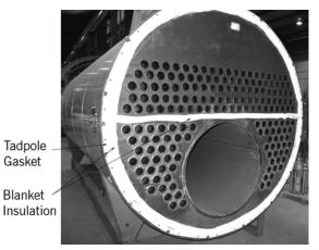
Figure 8-4 Gasket and Insulation — CB-LE
