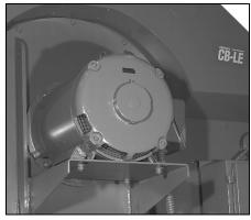
Figure 2-3 Fan Motor
