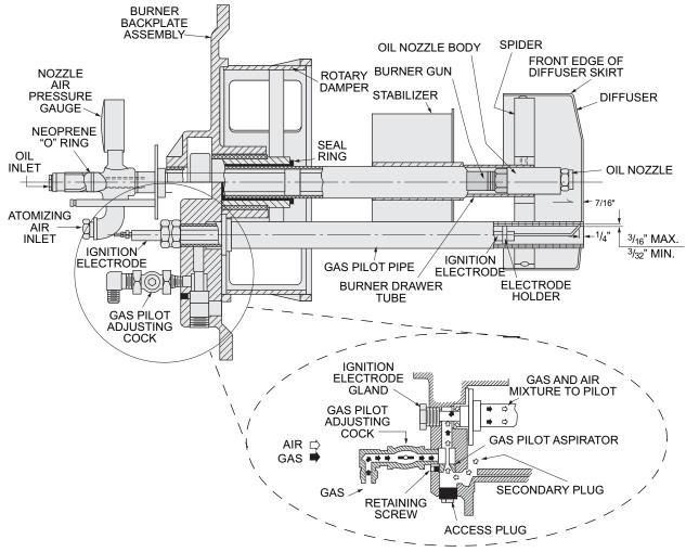
Figure 6-10 Burner Drawer with Gas Pilot
