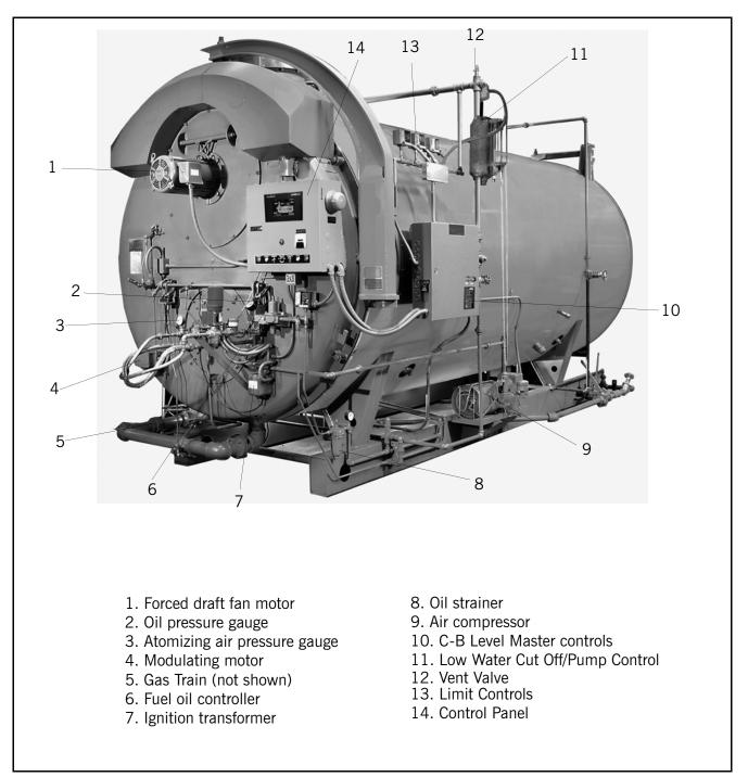
**Figure 1-2 CB-LE, Dual Fuel, Typical** (Components and component orientation may vary)
