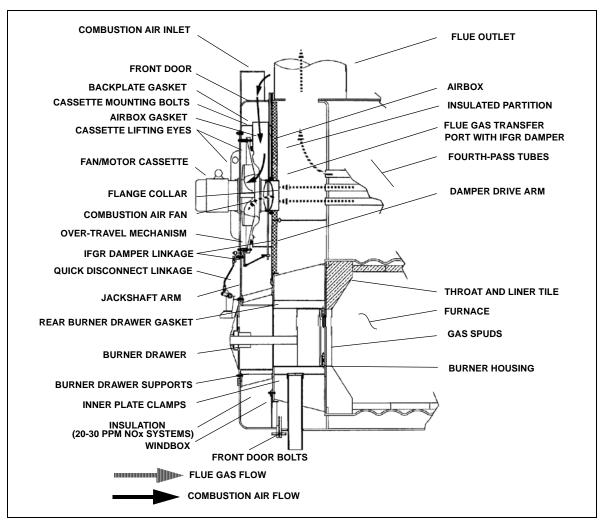
Figure 1-6 Induced Flue Gas Recirculation System, General Arrangement
