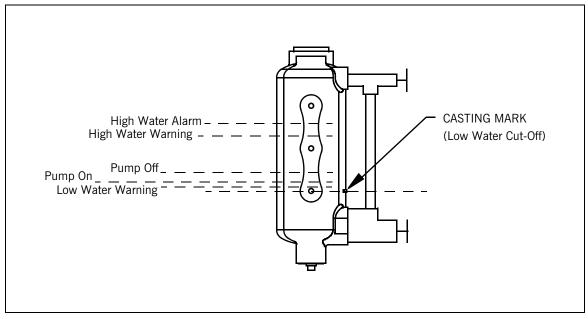
Figure 3-2 C-B Level Master water levels
