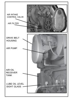
Figure 2-13 Belt Driven Air Pump (Model CB-OS)
