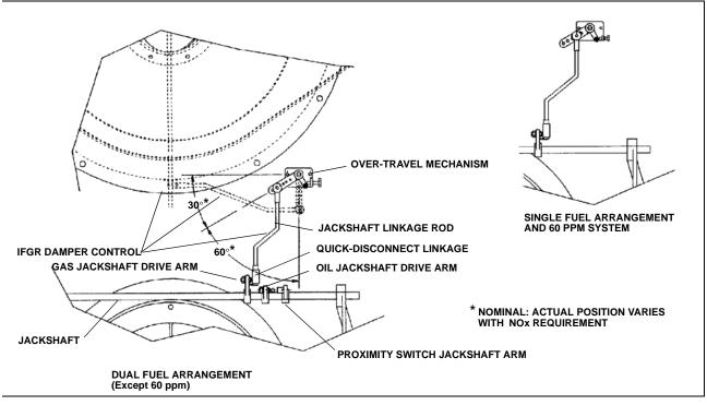
Figure 1-7 IFGR Damper Linkage
