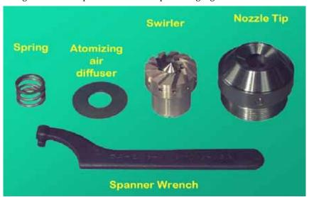
FIGURE 8-3. Standard Burner Nozzle Components
