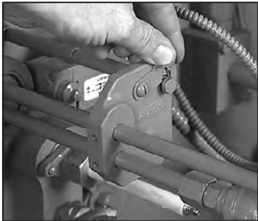
FIGURE 6-10. Figure 6-18 Oil Gun Locked Out
