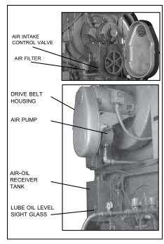
Figure 2-13 Belt Driven Air Pump (Model CB-OS)
