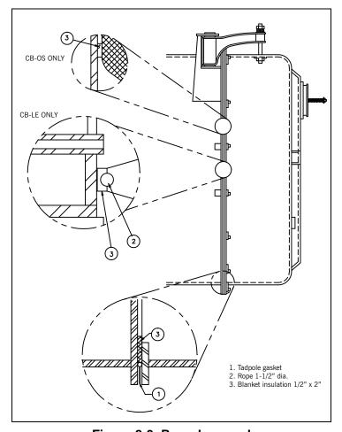
Figure 8-3 Rear door seal
