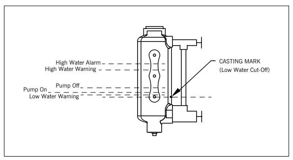
Figure 3-2 C-B Level Master water levels
