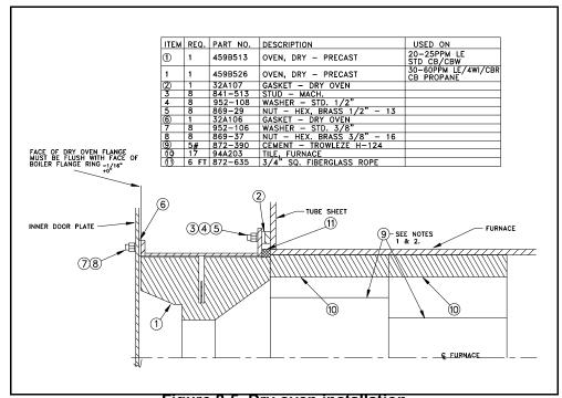
Figure 8-5 Dry oven installation
