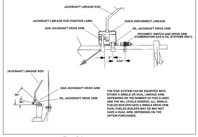
Figure 5-4 Jackshaft Linkage Settings
