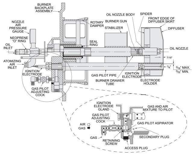
Figure 6-10 Burner Drawer with Gas Pilot
