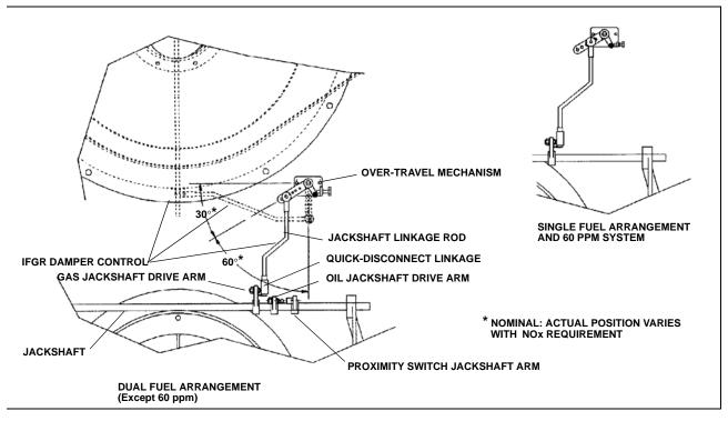
Figure 1-7 IFGR Damper Linkage
