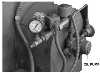
Figure 2-7: Mounted Oil Pump
