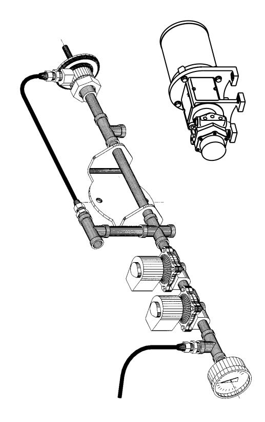
Figure 5-4: ProFire Burner Pressure Atomized with Remote Pump System
