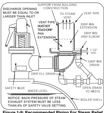
Figure 1-9: Recommended Piping For Steam Relief Valve (Not Furnished By Cleaver Brooks)
