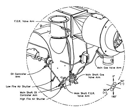
Figure 5-9: Burner Linkage Setup
