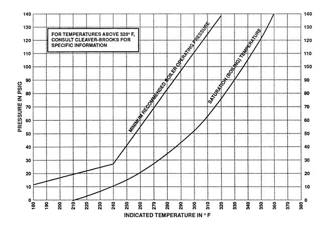
Figure 3-2: Internal Boiler Pressure
