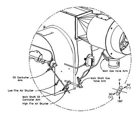
Figure 6-10: Initial Burner Linkage Setup
