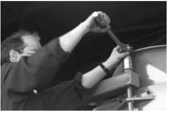
Figure: 8-6 Tighten Davit Nut
