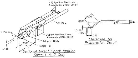
Figure 5-5: Direct Spark Electrode Setup
