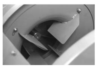
Figure 2-8: Air Box and Impeller
