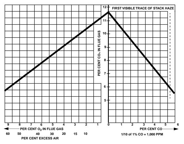
Figure 6-7: Flue Gas Analysis Chart for Natural Gas
