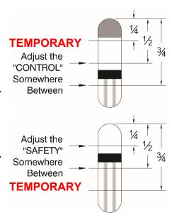
WARNING – Verify the Safety Valve (15) pressure rating on the valve itself before you begin. Never let the pressure reach this rating; if at any point the pressure reading on the Pressure Gauge (11) passes the desired "Safety" Pressure Switch (9) setting according to Table 2, shut down the generator, OPEN the Steam Outlet Valve (12), DECREASE the pressure setting on the "Safety" Pressure Switch (9), and restart at Step #4.
