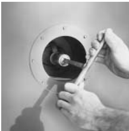
Removing hand hole assembly with a Tee Handle Wrench
