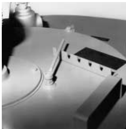
Secondary Air Adjustment 40-60 HP
