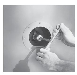
FIGURE 5 - REMOVE ASSEMBLY WITH TEE HANDLE WRENCH
