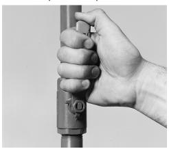
4. Open the water feed valve on boiler.
