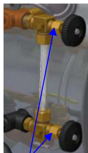
Loosen nuts at top and bottom of glass
