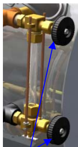
Close gauge glass valves (top and bottom).
