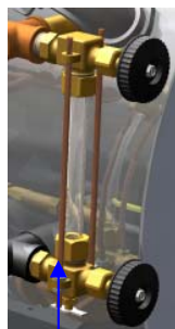
Remove gauge glass protector rods
