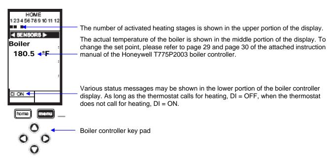
As soon as the temperature in the pressure vessel approaches the programmed set point temperature, the boiler controller will begin to step out heating stages.
