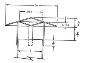
Figure 5, Stack Rain Cone
