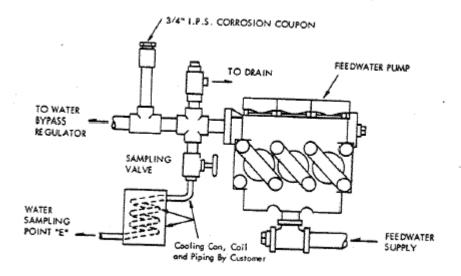
Figure 8, Typical Pump Piping
