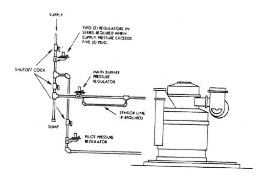
Figure 16, Gas Regulator Installation
