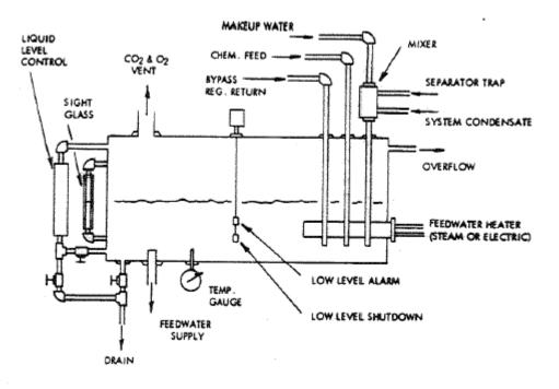
Figure 9, Recommended Feedwater Tank Design
