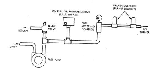
Figure 15, Fuel Oil Piping I.R.I. and F.M.
