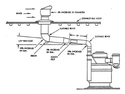
Figure 4, Stack Installation With Horizontal Run
