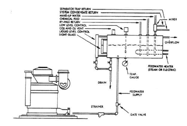
Figure 7, Water Tank Installation (See Page 35)
