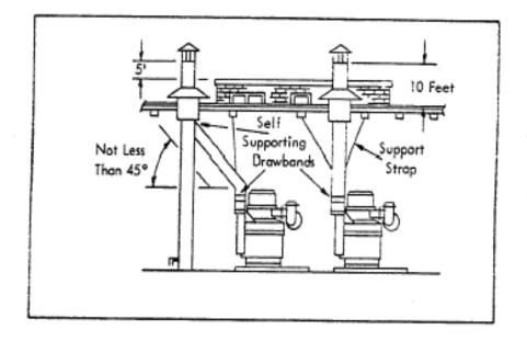
Figure 2, Recommended Stack Installation
