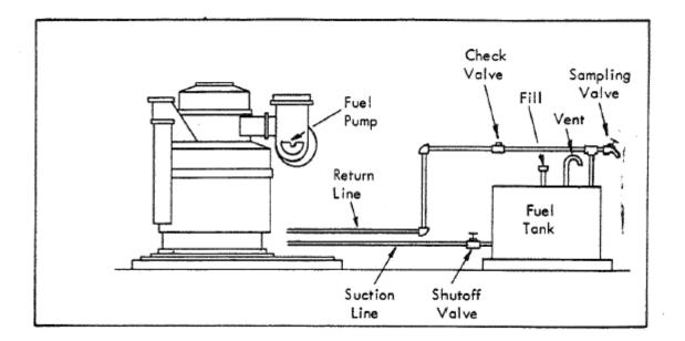
Figure 14, Fuel Tank Installation
