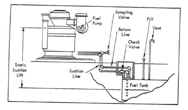
Figure 13, Underground Fuel Tank Installation
