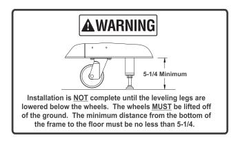
5. Extend mounting legs further as needed until the boiler is level. Check level, front to back as well as side to side. Measure level on top panel of boiler NOT across the heat exchanger, since it is intentionally tilted within the boiler enclosure.
