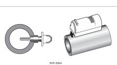
1/2" NPT -4" long Immersion sensors standard. Optional strap on sensors available in Replacement Part section.
