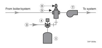
Figure 12 Expansion tank piping — closed-type expansion tank
