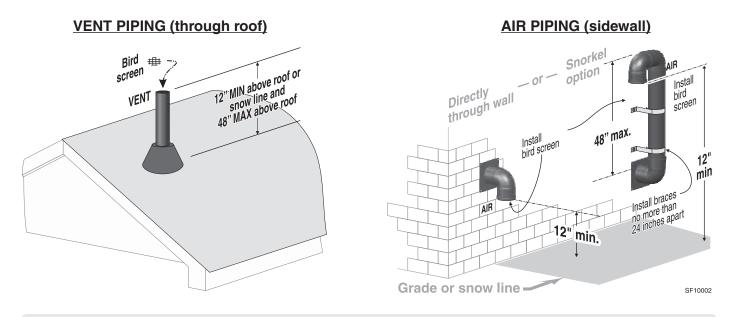
**AWARNING** Multiple boiler applications — Space vents minimum 6 inches apart. Space air terminations minimum 6 inches apart.
