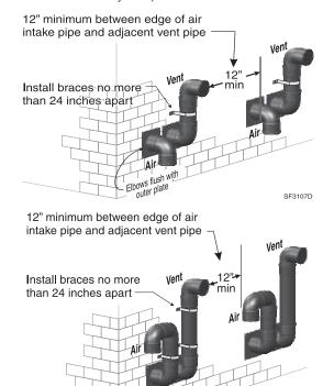
Figure 33 DIRECT VENT — sidewall termination assembly.
