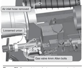
Figure 78 Cover plate up for burner removal and replacement
