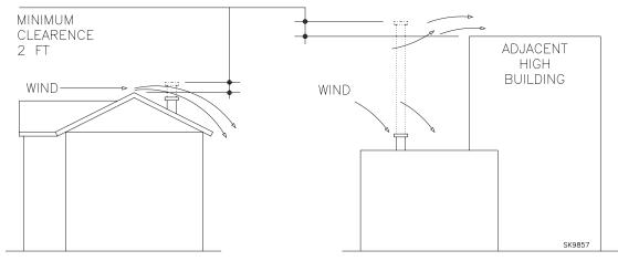
**NOTE:** Correct chimney design is shown by dotted lines. Incorrect chimney design, as shown by the solid lines, may result in down-drafts.
