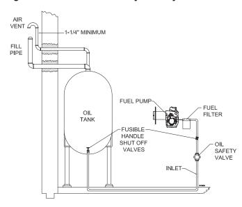
Figure 9. - Outside Buried Tank-Lift System
