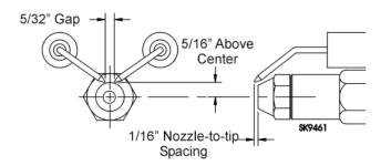
The Dimensions shown below are for use with L2 heads and M series air tube combinations ending with an 'N' suffix (example: AFG70MDAQ $\mathbf{N}$ )
