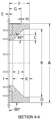
FIGURE 2-3. E-Series Refractory Dimensions
