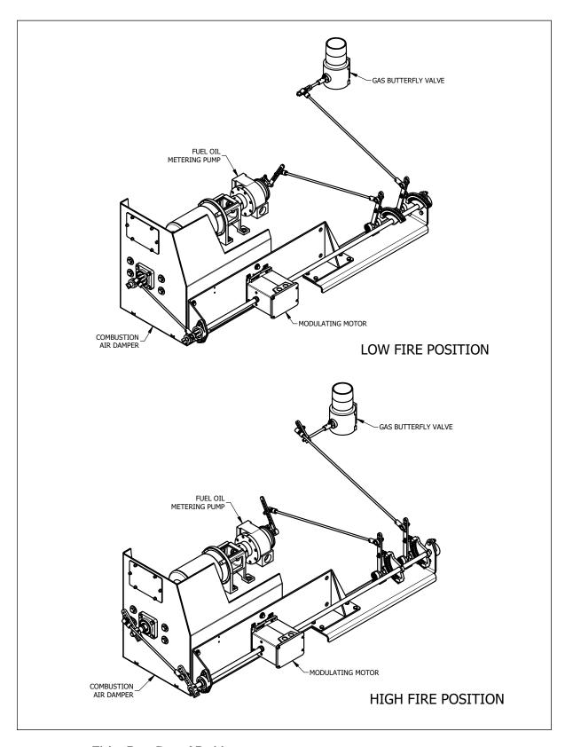
FIGURE 4-2. Firing Rate Control Positions
