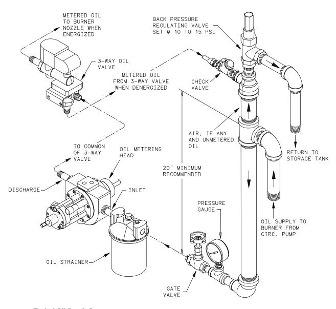
FIGURE 2-5. Typical Oil Supply Loop
