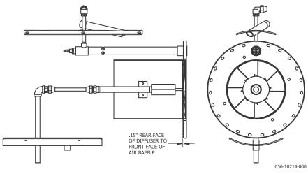
FIGURE 4-11. Drawer Assembly for (VG) Gas Only (V120-168) - Firetube
