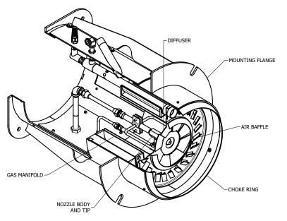
FIGURE 1-2. Burner Housing (Firetube Applications)
