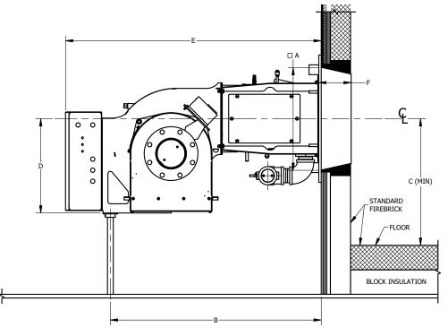
FIGURE 2-3. Standard Configuration for Watertube/ Cast Iron Boiler
