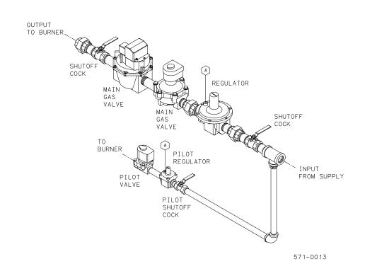
FIGURE 1-10. Typical Gas Train for LHO System (V13-34)
