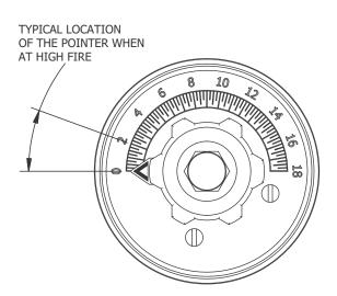
FIGURE 4-23. Oil Metering Adjustment Knob
