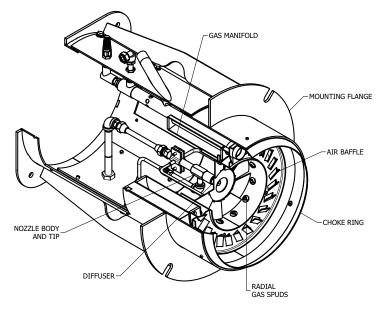
FIGURE 1-1. Burner Housing (Watertube Applications)
