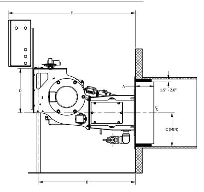
FIGURE 2-2. Inverted Configuration for Firetube Boiler
