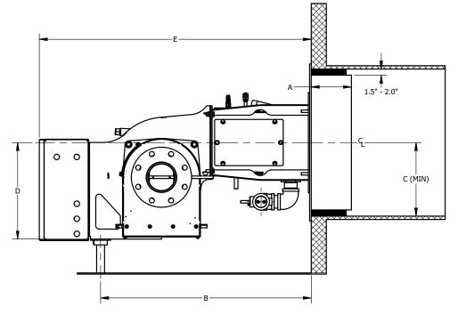
FIGURE 2-1. Standard Configuration for Firetube Boiler
