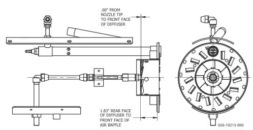
FIGURE 4-15. Drawer Assembly for (VLG) Gas/Oil (V13-34) - Watertube/ Cast Iron
