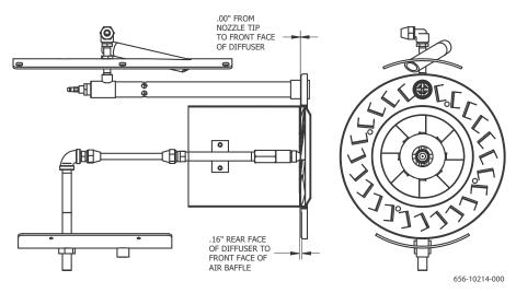
FIGURE 4-10. Drawer Assembly for (VLG) Gas/Oil (V60-110) - Firetube
