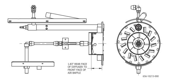
FIGURE 4-13. Drawer Assembly for (VG) Gas Only (V13-34) - Watertube/ Cast Iron
