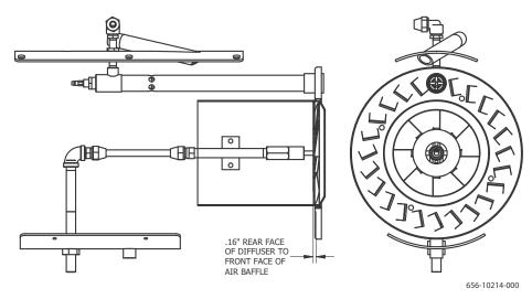
FIGURE 4-9. Drawer Assembly for (VG) Gas Only (V60-110) - Firetube
