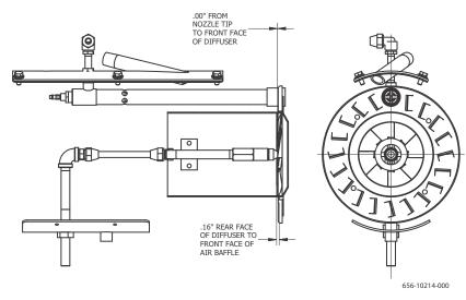
FIGURE 4-8. Drawer Assembly for (VLG) Gas/Oil (V35-55) - Firetube
