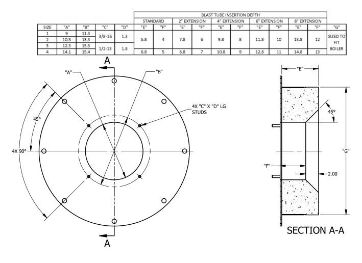
FIGURE 2-5. V Series Refractory Dimensions
