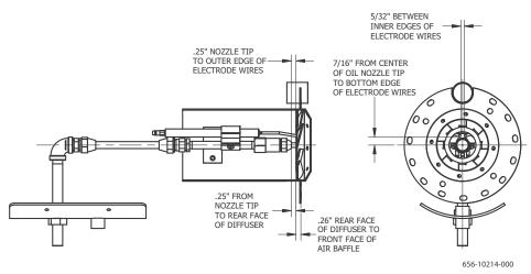
FIGURE 4-4. Drawer Assembly for (VL) Oil Only (V13-34) - Firetube
