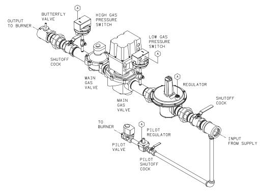
FIGURE 1-12. Typical Gas Train for LHO/LHL Systems (V35-63) & Full Modulation Systems (V35-168)
