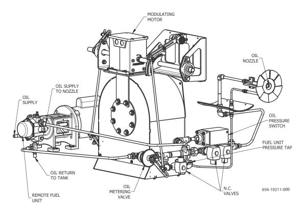
FIGURE 1-8. Full Modulation Oil System with a Remote Pump (V60-168)
