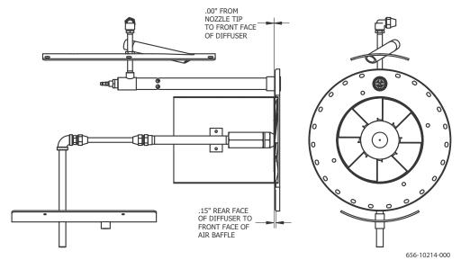
FIGURE 4-12. Drawer Assembly for (VLG) Gas/Oil (V120-168) - Firetube
