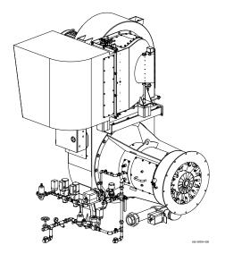
FIGURE 8-1. General Layout of the Burner
