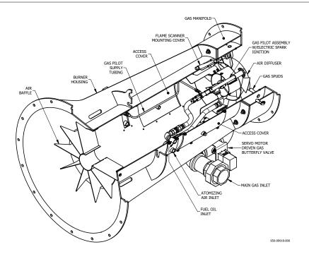
FIGURE 1-1. Burner Housing
