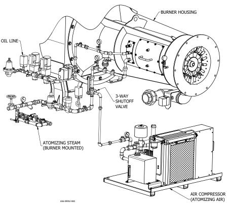
FIGURE 7-1. Steam Atomizing System
