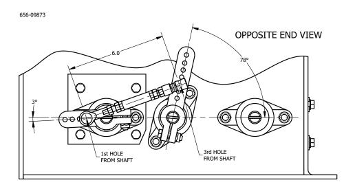
FIGURE 4-1. Firing Rate Control Positions
