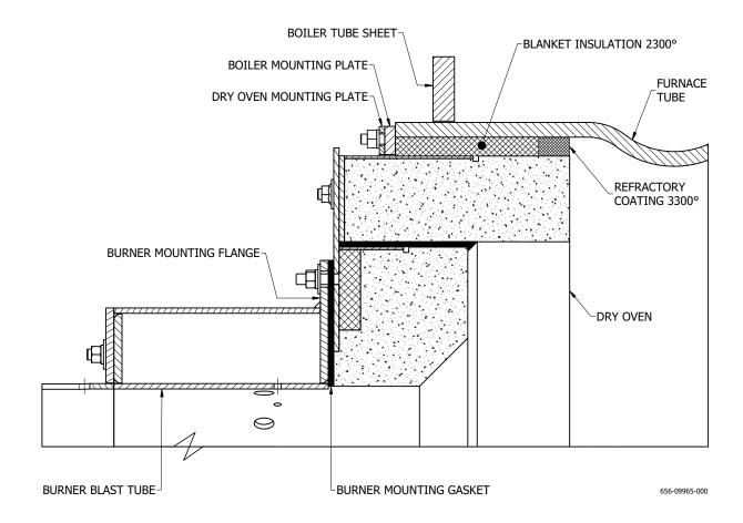
FIGURE 2-1. Dry Oven Installation
