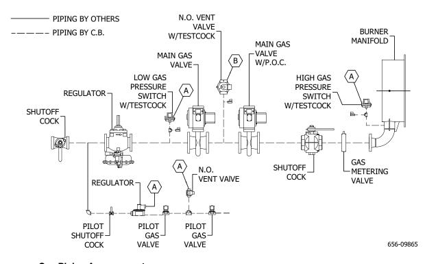
FIGURE 2-4. Gas Piping Arrangement
