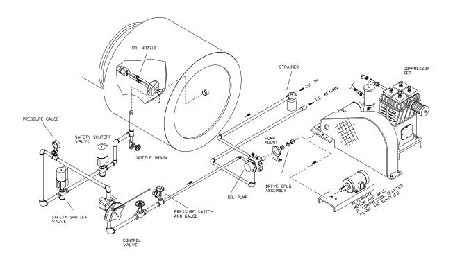
Figure 7.3: Typical #2 Oil Train Small Pump
