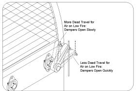
Figure 9.3: Inlet Air Damper Adjustment
