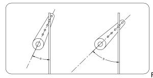
Figure 9.5: Linkage Modification
