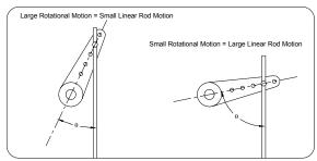
Figure 9.2: Linkage Arm Modification
