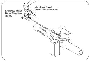
Figure 9.4: Fuel Valve Modification
