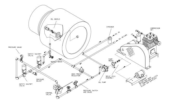
Figure 7.3: Typical #2 Oil Train Large Pump
