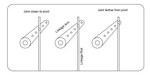
Figure 9.1: Linkage Joint Adjustment
