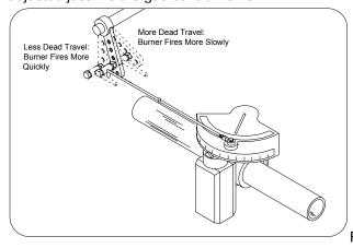
Figure 9.4: Fuel Valve Modification
