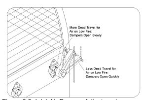
Figure 9.3: Inlet Air Damper Adjustment
