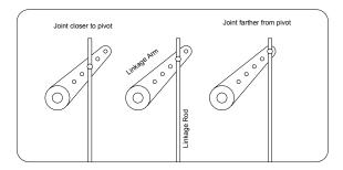
Figure 9.1: Linkage Joint Adjustment
