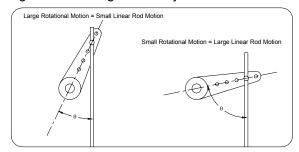
Figure 9.2: Linkage Arm Modification
