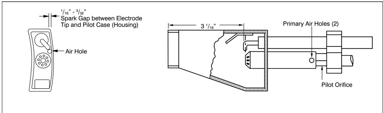
For C5B, C6, C7 and C8 Pilot Ignition Electrode Adjustment, see Figure 37, page 37.
