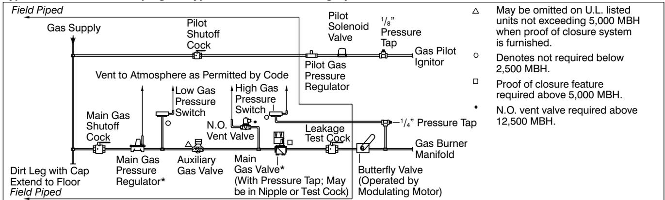
\* On some burner models at inputs below 2500 MBH a combination pressure regulator/automatic gas valve may be used in place of the separate main gas pressure regulator and main gas shutoff valve shown in Figure 8 and 9 above. For specifics on your burner refer to the gas piping diagram supplied with the burner.
