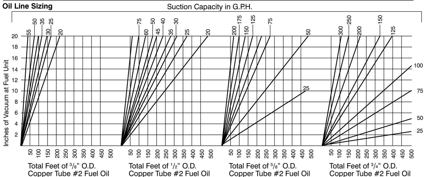
1. Check oil pump *GPH Suction Capacity* shown in Table 6.
