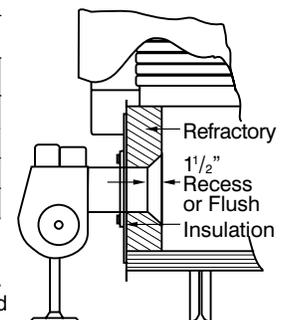
Note: The above minimum dimensions are recommended. If boiler dimensions are less, consult with factory. All burners set through refractory with sleeve to allow field removal. Unlined space between sleeve and burner blast tube closed with non-asbestos high-temp rope or KA-O-Wool.
