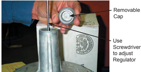
Figure E – 9 Main Gas Pressure Regulator Adjustment
