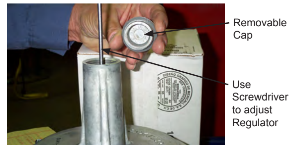
Figure E – 7 Main Gas Pressure Regulator Adjustment
