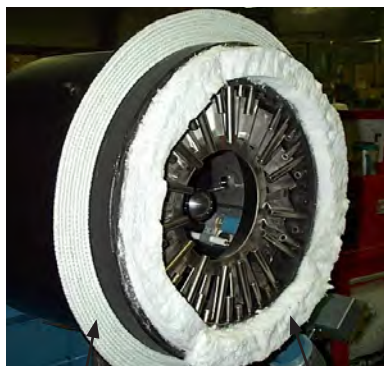
Figure C-2 Ceramic Blanket and Rope Gasket
