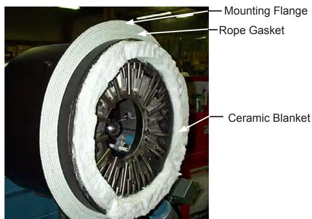
Figure B-13 Gas Manifold
