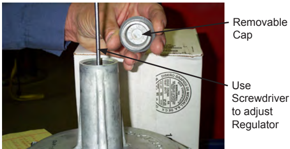
Figure E – 9 Main Gas Pressure Regulator Adjustment
