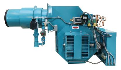
The new "SC" series burner from Webster Combustion combines the reliable and rugged burner technology Webster is known for with a new, patented staged-combustion firing head. This new offering allows the user to operate with low emissions without the cost and expense of external Flue Gas Recirculation
