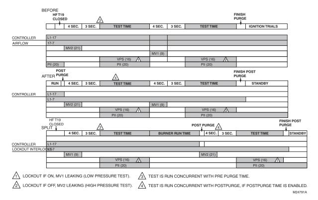
Fig. 10. CB780E/CB784E Relay Module operation, Valve Proving test options.
