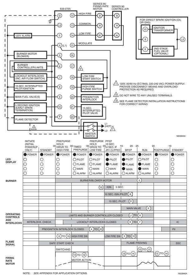
Fig. 8. Typical wiring subbase and sequence for the CB780E/CB784E, without Valve Proving.
