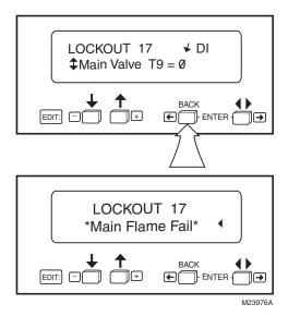
Fig. 43. BACK push-button function.
