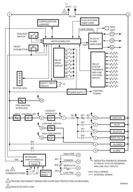
Fig. 7. Internal block diagram of the CB780E/CB784E (see Fig. 8-13 for detailed wiring instructions).
