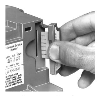
Fig. 15. Purge card installation.
