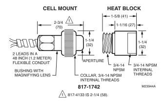
Fig. 6. Infrared detector, mounting dimensions in inches (mm).
