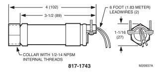
Fig. 5. Ultraviolet detector, mounting dimensions in inches (mm).
