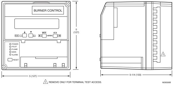
Fig. 2. Mounting dimensions of CB780E/CB784E Relay Module and 833-2725 Subbase, in inches (mm).
