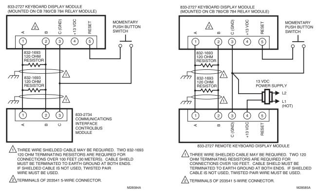
Fig. 11. Wiring the Keyboard Display Module with Communications Interface ControlBus Module.
