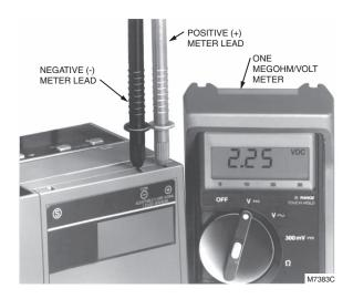
Fig. 47. Flame signal measurement.
