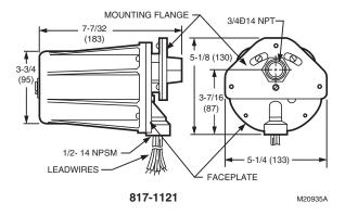
Fig. 4. Ultraviolet Self-Check detector, mounting dimensions in inches (mm).
