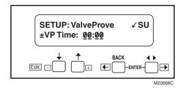
Fig. 26. Valve Prove time screen.
