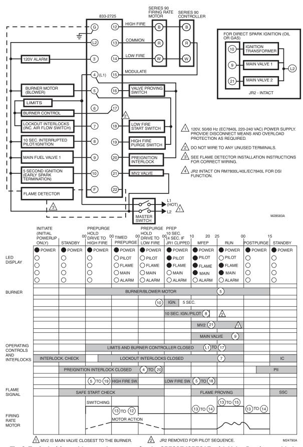
Fig. 9. Typical wiring subbase and sequence for the CB780E/CB784E, with Valve Proving enabled.
