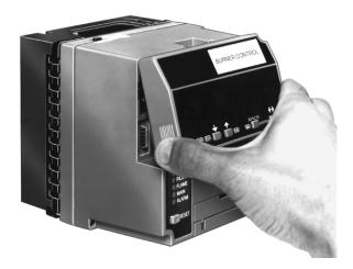
Fig. 16. Keyboard Display Module installation.
