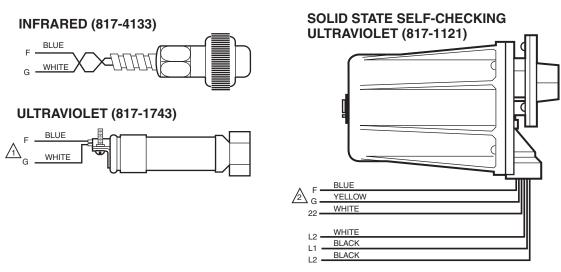
FLAME DETECTOR LEADS ARE COLOR CODED. THE BLUE LEAD MUST BE CONNECTED TO THE F TERMINAL AND THE WHITE MUST BE CONNECTED TO THE G TERMINAL. THE UV SENSING TUBE IS POLARITY SENSITIVE. REVERSING THE LEADS EVEN MOMENTARILY CAN DAMAGE OR DESTROY THE UV TUBE.
