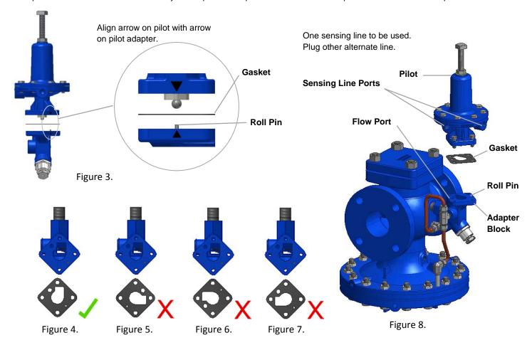
When installing pilot on opposite side of the main valve, make sure the pilot is installed in the proper orientation. The arrows on the pilot adapter and the pilot should be aligned. See figure 3.
